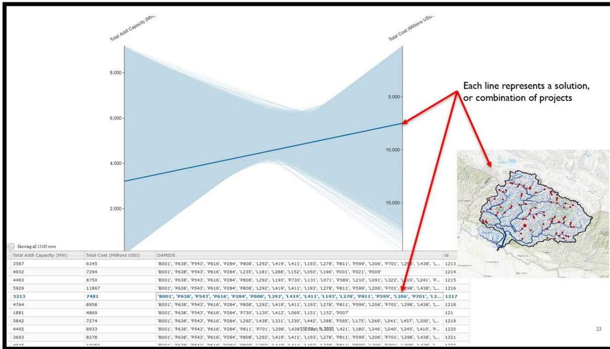
Each of the vertical axes in the plot correspond to a metric. Where each line crosses an axis represents the solution's value for that metric. Figure 2 shows a highlighted solution and its values for installed capacity (MW) and total cost (millions of US dollars). The values for the solution are also available in the linked table below the parallel plot.
